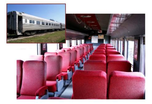
The 106 was built by the Budd Company in 1939 for the Seaboard Air Line Railroad, the first in lot number ZA146. This car was used in SAL's Silver Meteor trains as a 56 seat coach and was originally numbered 6203. The number was changed to 5607 upon the merger with the Atlantic Coast Line Railroad to form Seaboard Coast Line. The car retained that number through the transfer to and use by Amtrak.
